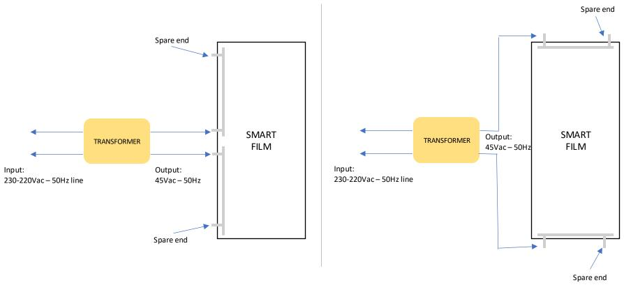
**NOTE:** Each busbar has two ends. Wire can be joined on only one of them. The other one end is a spare end.
